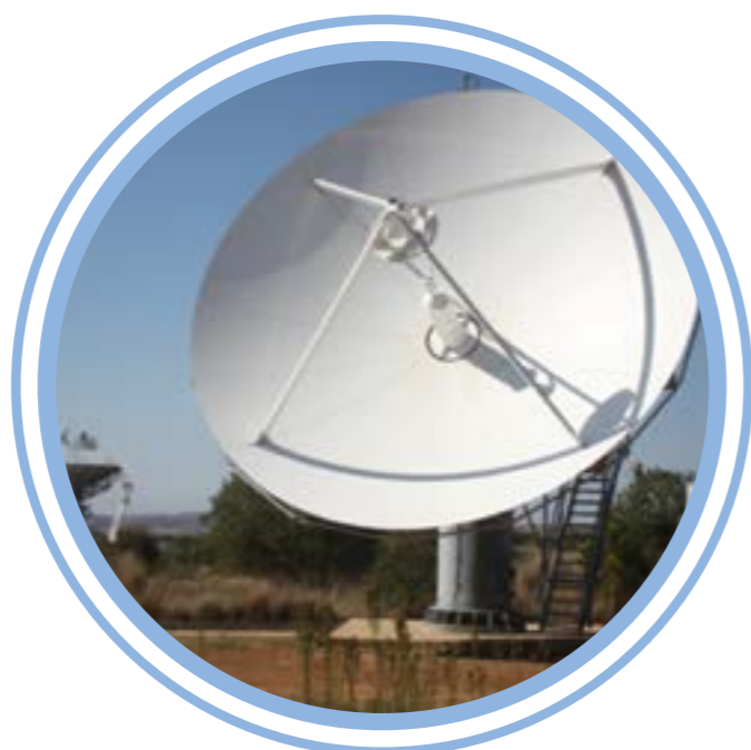
The new KU-DBS band antenna in the foreground and the almost-completed C-band in the background, on the left
